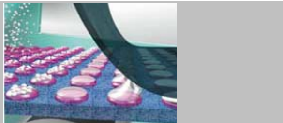
Behavior of the coating dots during fusing as a function of the coating process
